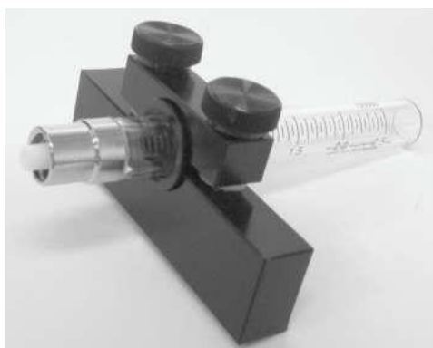
Figure 12.13: Syringe clamp with syringe
