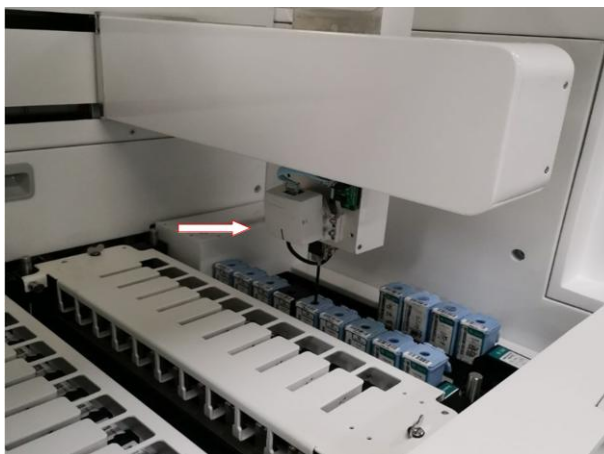
Figure 3.4: Robotic arm, the arrow indicates the scanning module
